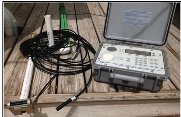
Figure 15. Vemco VR-100 hand-held sonic receiver (right), with VH110 directional hydrophone (left) and VH165 omnidirectional hydrophone (center).
